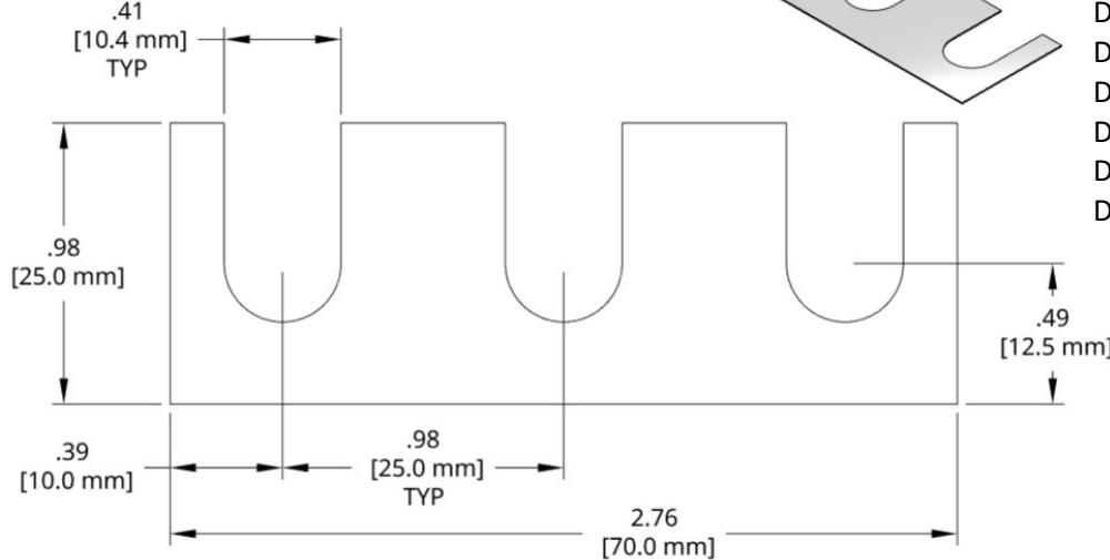
Full Hard 1010 steel shim stock. Black Oxide finish on -M050, -M100 and -M200 thickness shims.
