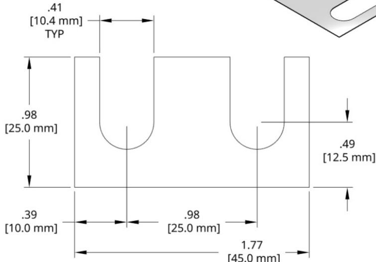
Full Hard 1010 steel shim stock. Black Oxide finish on -M050, -M100 and -M200 thickness shims.
