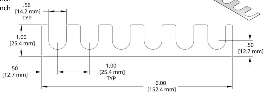
Full Hard 1010 steel shim stock. Black Oxide finish on -M050, -M100 and -M200 thickness shims.
