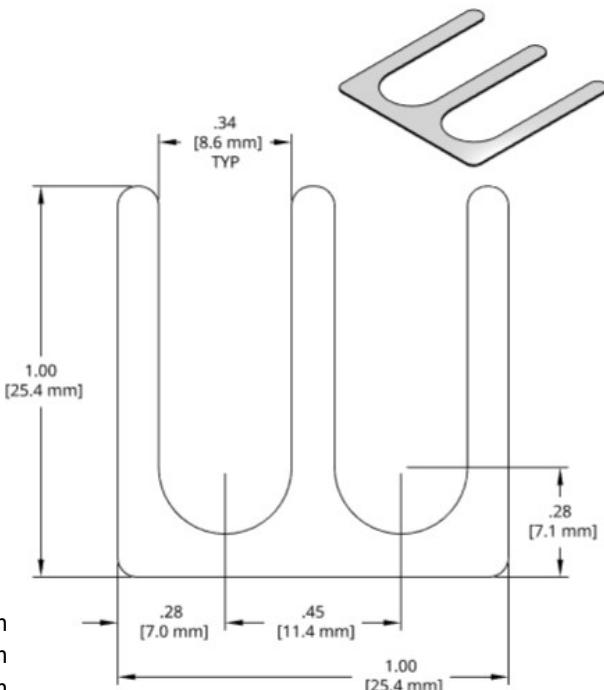
Full Hard 1010 steel shim stock. Black Oxide finish on -M050, -M100 and -M200 thickness shims.
