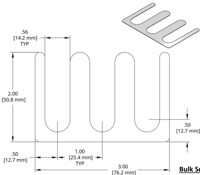
Full Hard 1010 steel shim stock. Black Oxide finish on -M050, -M100 and -M200 thickness shims.
