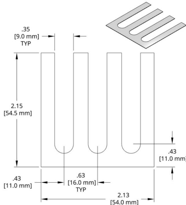
Full Hard 1010 steel shim stock. Black Oxide finish on -M050, -M100 and -M200 thickness shims.
