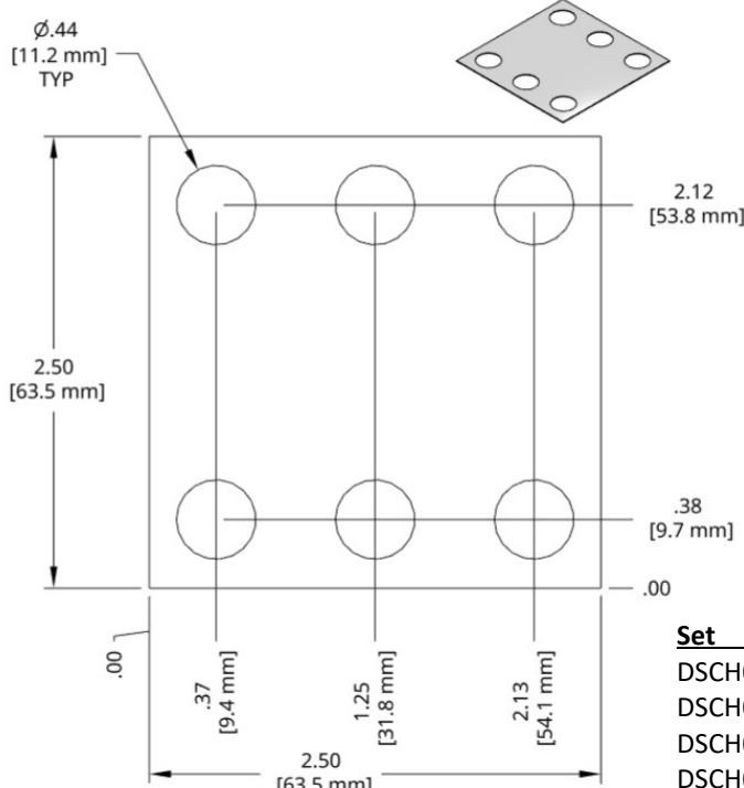
Full Hard 1010 steel shim stock. Black Oxide finish on -M050, -M100 and -M200 thickness shims.
